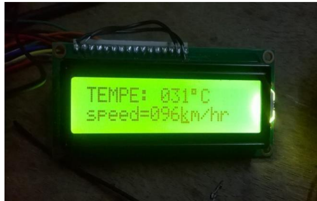
Fig.2 Real time Speed on LCD
